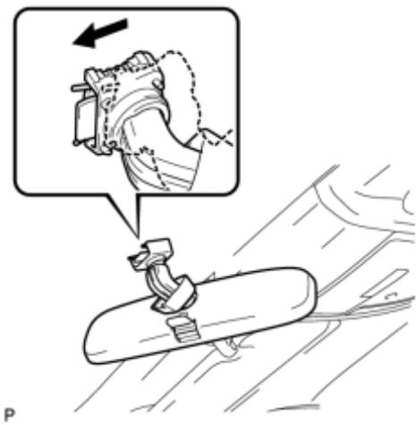
(a) Install the inner rear view mirror as shown in the illustration.
