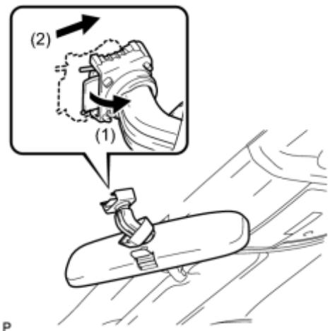
(b) Remove the inner rear view mirror as shown in the illustration.
