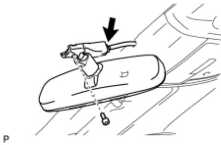
(1) Using "TORX" socket wrench (T20), install the inner rear view mirror with the screw.
